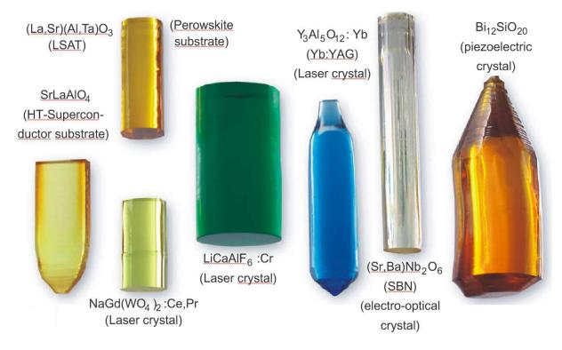
Fig. 1: Oxide and fluoride crystals prepared at the IKZ (selection).
